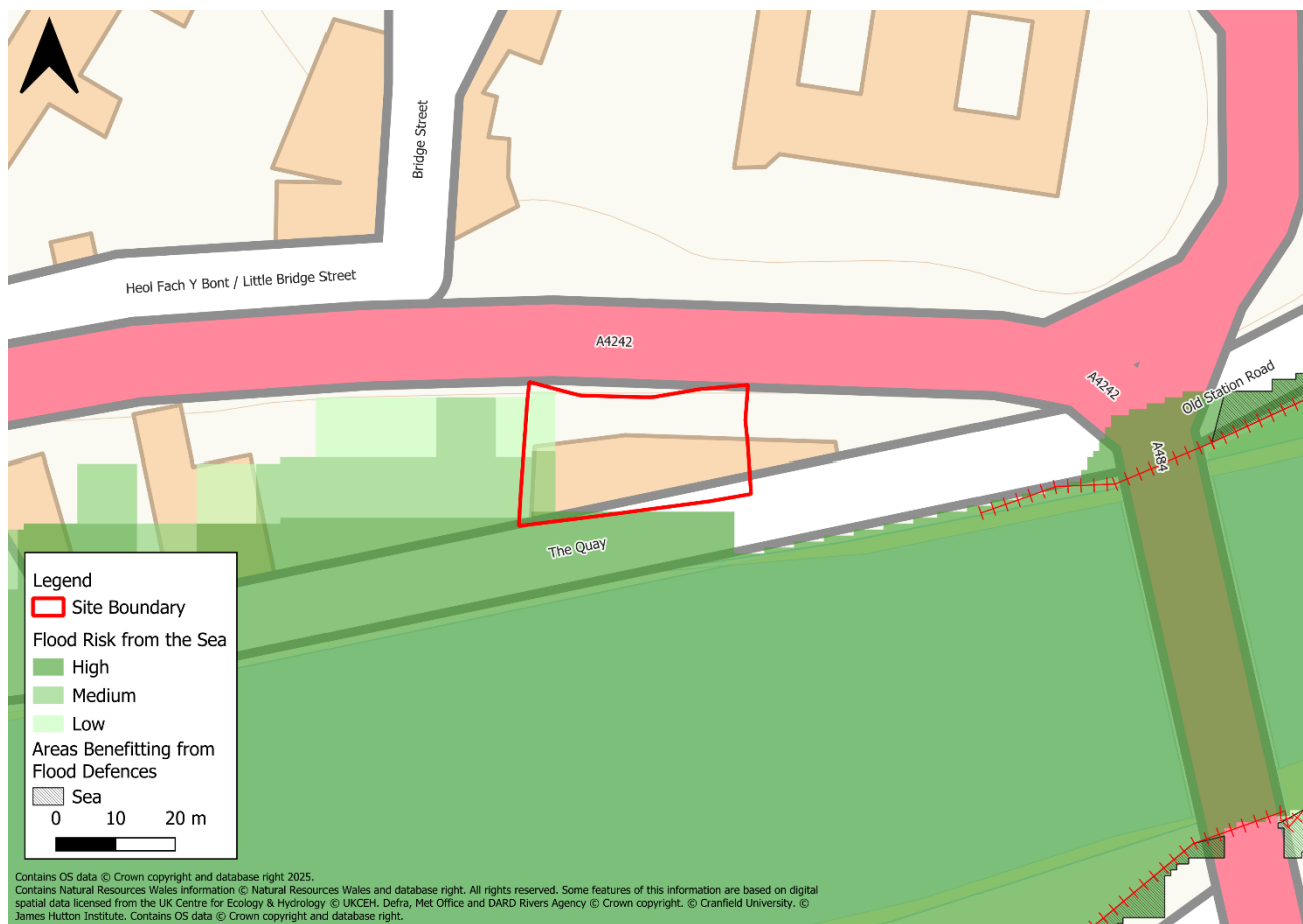
Figure 4-2 FRAW - Flood Risk from the Sea
